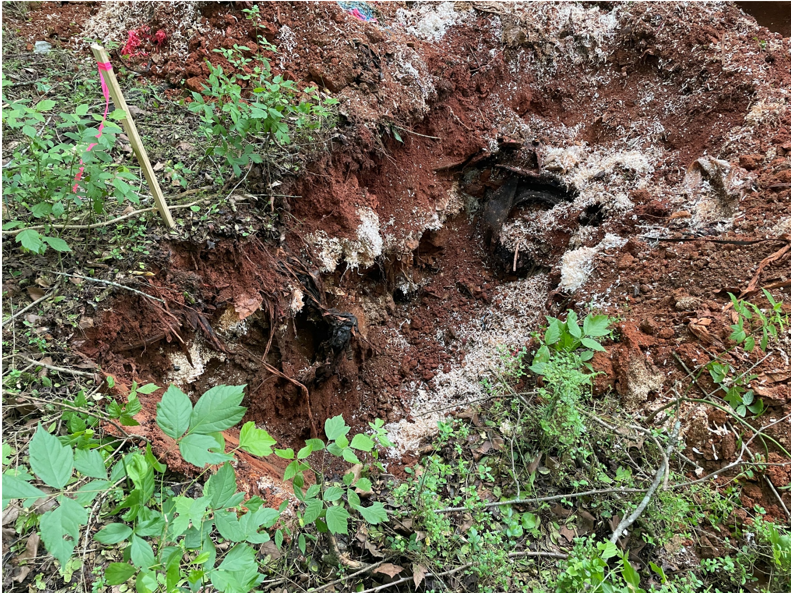
Test Pit #12 - debris fill encountered to a depth of 7 feet bgs
